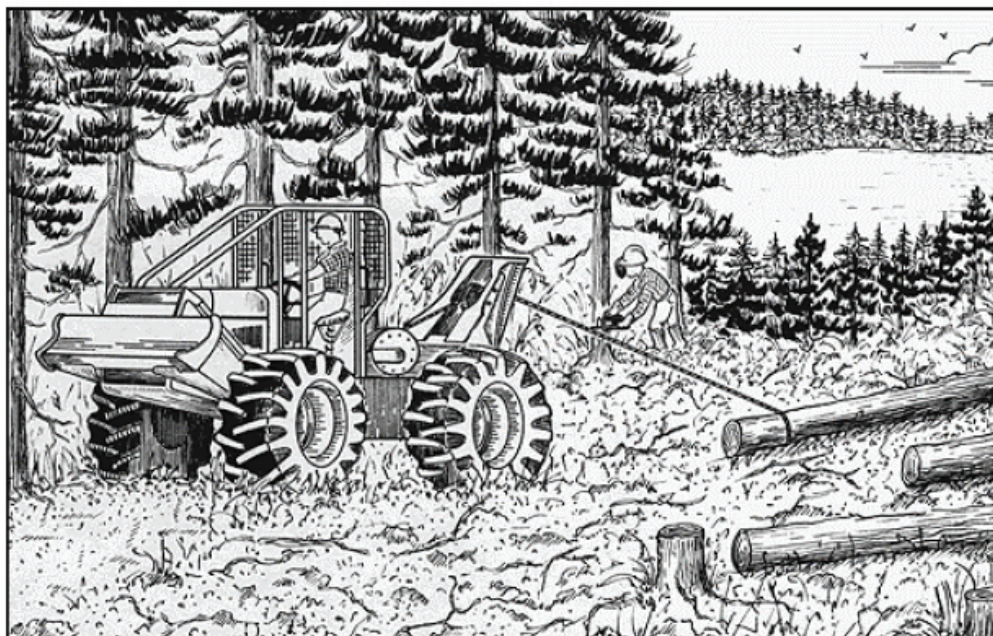
Figure 5. Fell trees away from water to avoid debris loading. The use of extra-long winch cables allows the surface vegetation to remain intact, an important consideration on sensitive soils.
