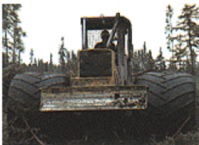
Figure 4. Fine textured soils, and deep, wet organic soils are more prone to soil disturbance than other soils. High flotation harvesting equipment should be used on sites where the potential for erosion, rutting, and compaction is high.
